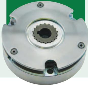
The thin spring-engaged power-off brake is electromagnetically released and has a relatively thin profile compared to normal spring-engaged brakes. This feature -- along with being RoHS compliant -- makes them a perfect candidate for a variety of applications while providing a good torque-to-size ratio.
