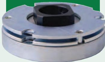
The ultra-thin spring-engaged, electromagnetic power-off brake offers a low backlash hub and is the thinnest profile power-off brake available in the market. The short package size allows the brake to be easily mounted to the front or rear of a motor. Equipped with PWM controller to reduce heat and save energy for continuous duty applications. The UTSEB is also RoHS compliant.
