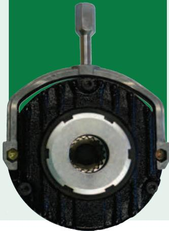
The motor spring-engaged power-off brake is designed to easily mount to a motor or frame. The brake includes a manual release lever which provides an override in the absence of power and a dust cover to help keep the friction surface free of debris. A torque adjustment collar also allows the torque to be manually adjusted based on the application.
