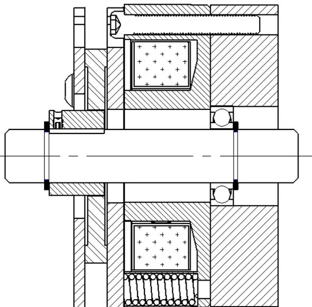
Shown here is a model SEB mounted to a front shaft hub and rear mounting plate. The rear mounting surface is to be flat and perpendicular to rotating shaft within 0.003" total.
